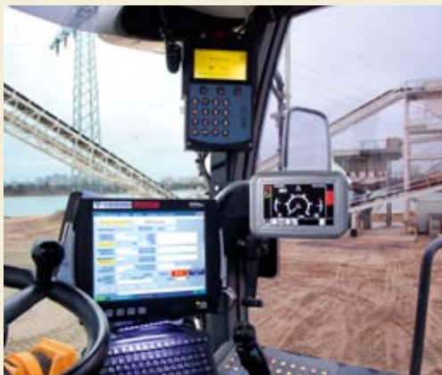
Wheel Loader Terminal with legal-for-trade wheel loader scale and ticket printer
